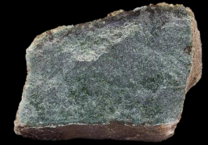
Holomelanocratic, ultramafic, aphanitic. Typically Komatiites
