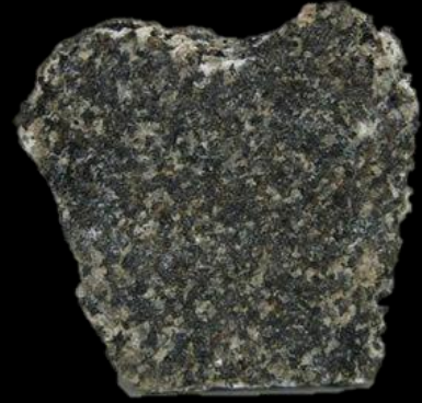
Melanocratic, mafic, phaneritic. Typically gabbros
