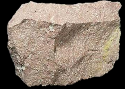
Leucocratic, felsic, aphanitic Typically rhyolites
