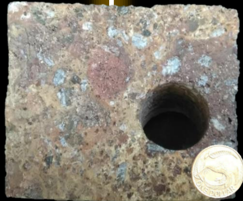
Pyroclastic rock. \phi : 47%. k: 798 mD
