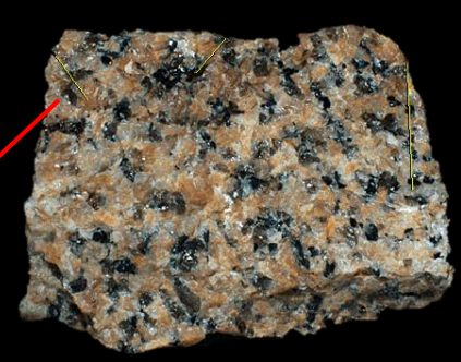
Leucocratic, felsic, phaneritic. Typically granites
