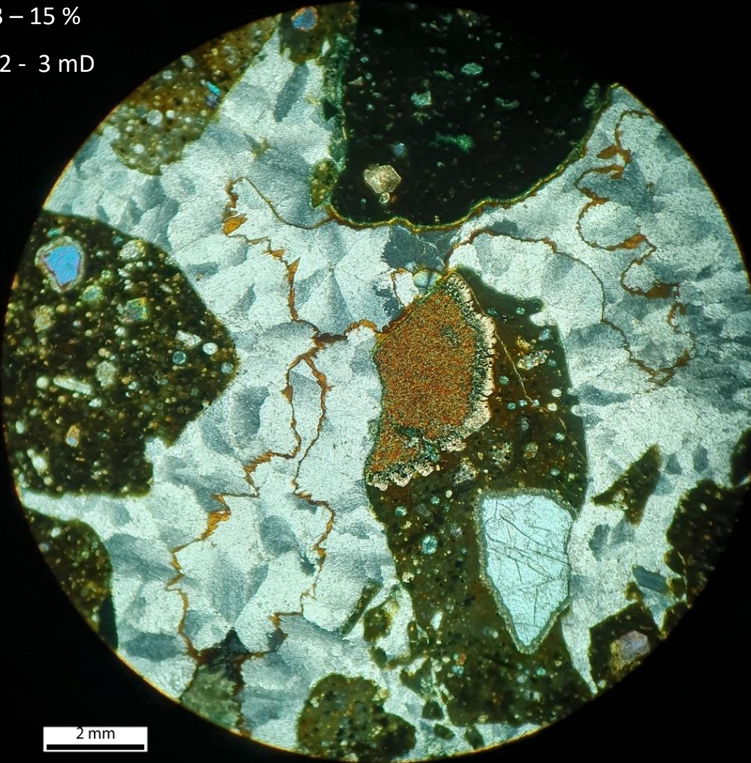
Cemented lapilli tuff
