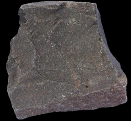
Melanocratic, mafic, aphanitic. Typically basalts
